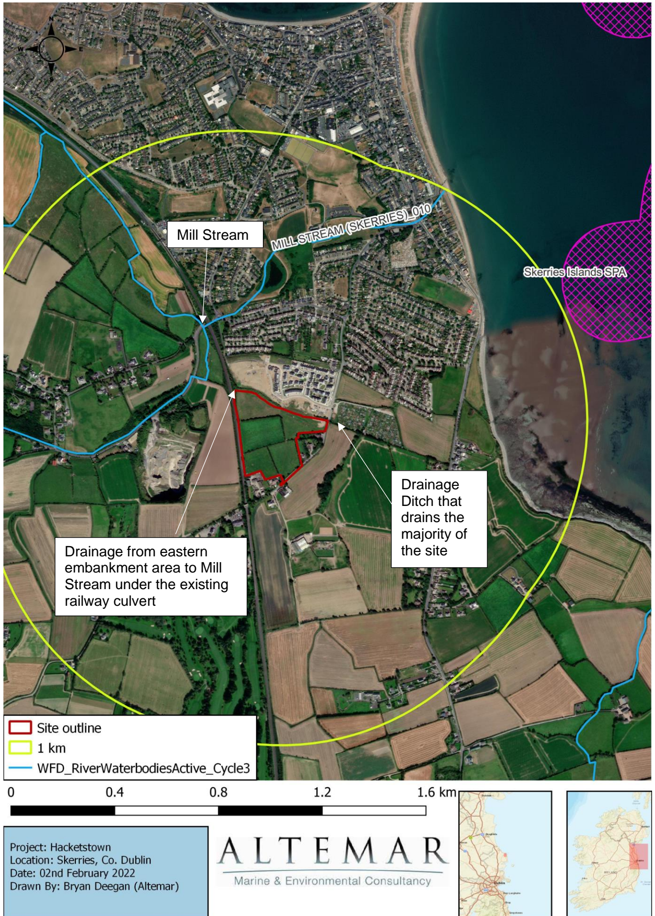
Figure 5.5 – Watercourses (drainage ditch on site entering the Mill Stream and Irish Sea directly).
